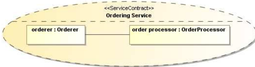
Figure 2: Example ServiceContract structural diagram
